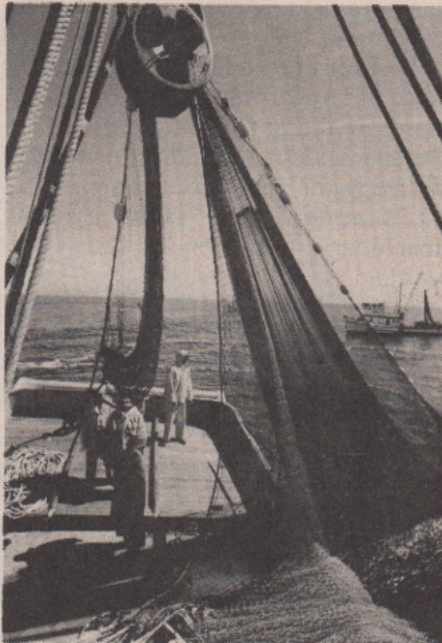
The crew of the El Dorado runs one end of the seine through the power block. Crewmen stack it as it's pulled, handling the net only once where with a lampara, the net must be handled twice—first to pull it in, then to restack it.
